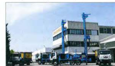
Below: M.I.45 rig with 45t pull-back and 2,350kg/m of torque for Ethiopia
