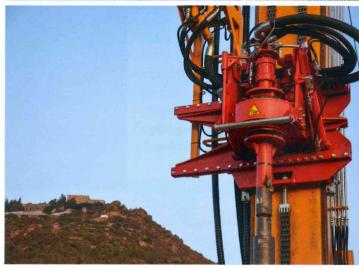
A Massenza MI55 in Cyprus for drilling wells to depths of up to 800 m with particularly complex geological formations
