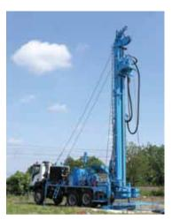
All drilling rigs are completely hydraulically driven and are very robust
